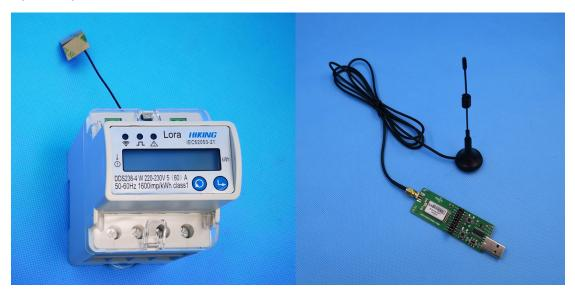
The meter is designed to measure single phase two wire AC active energy variable parameter like residential, utility and industrial application. It has remote read communication port RS485 and Lora wireless. It is a long life meter with the advantage of high stability, high over load capability, low power loss and small volume.
